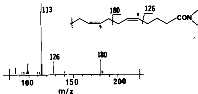
FIG. 3. Partial mass spectrum of 25-methyl-5,9-heptacosadienoic acid pyrrolidide showing the typical fragmentation peak at m/z 180.
